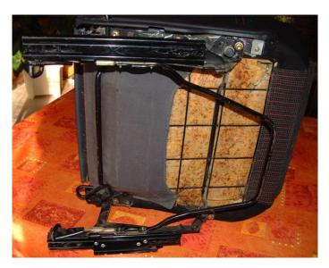
With the seat as above remove the plastic outer trim piece (3 Philips screws) and then take of the seat runner -4 Torx screws (2 per side).
