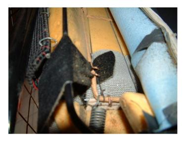
We will tackle the vinyl first, this bottom fixing is wired, remove the hog rings and fold it back to reveal the attaching and tension points for the bottom sections of the squab bolster covers. Remove these.
