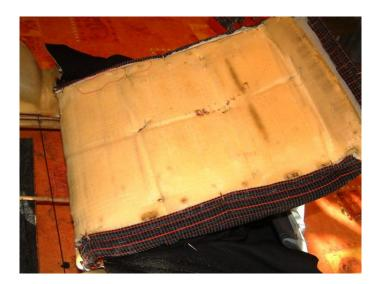
Start at the bottom first and as you remove the hog rings lift the cover as you go.
