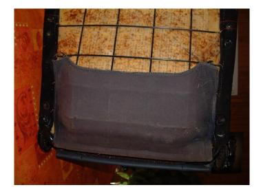
Held by hog rings either side attaching it to the wire seat frame. Pull this back to reveal the second transverse (wired) fixing point.
